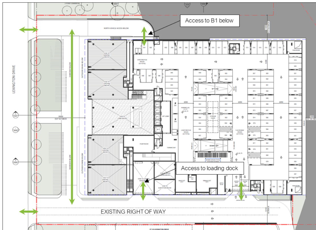
Figure 2.3: Proposed site access arrangements
